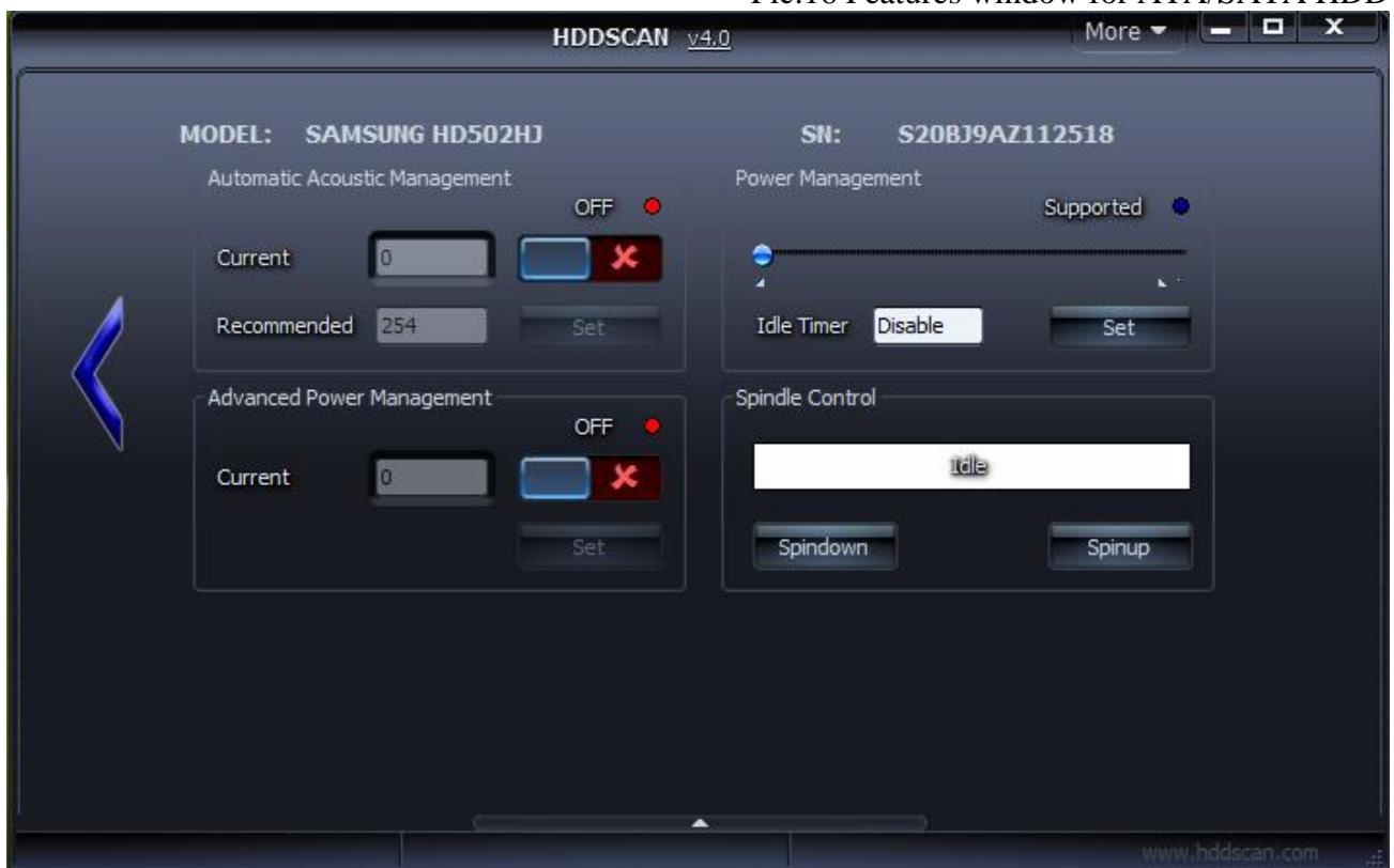
Pic.16 Features window for ATA/SATA HDD
